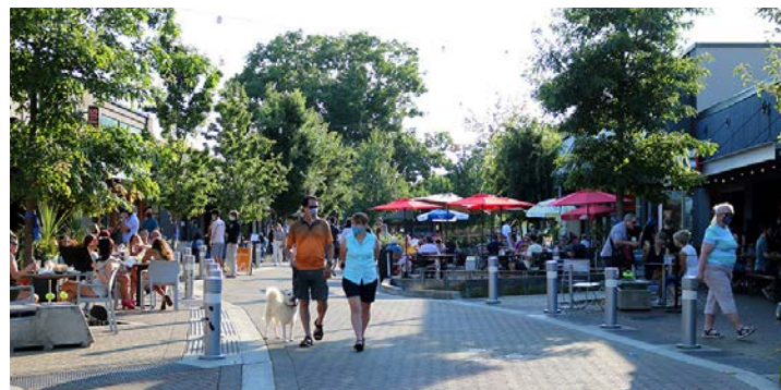
Permeable interlocking concrete pavement allows for efficient stormwater management, while creating an accessible environment. Image Source: City of Kirkland, WA
