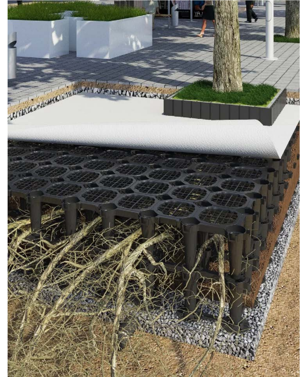
Visualization showing root growth within a modular soil cell. Image Source: Citygreen Urban Landscape Solutions
