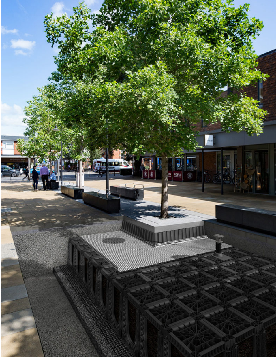
Visualization showing a modular soil cell underneath a tree planting. Image Source: GreenBlue Urban
